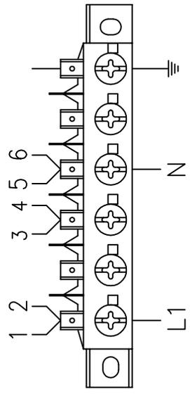
230V/3/50Hz 3800W 9.6A main cable 4x2.5mm<sup>2</sup>
