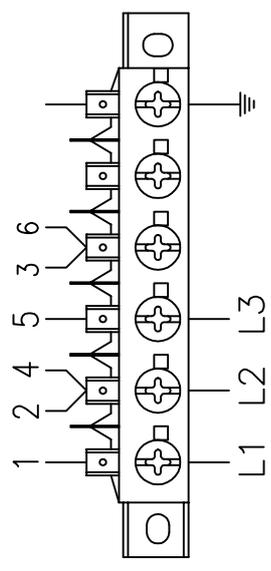
400V/3N/50Hz 2200W 3.2A main cable 5x1.5mm<sup>2</sup>
