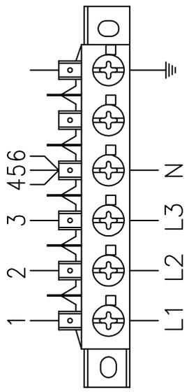
230V/50Hz 5450W 23.7A main cable 3X4mm<sup>2</sup>
