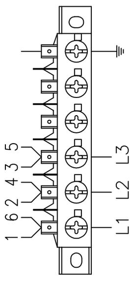
400V/3N/50Hz 3800W 5.5A main cable 5X1.5mm<sup>2</sup>
