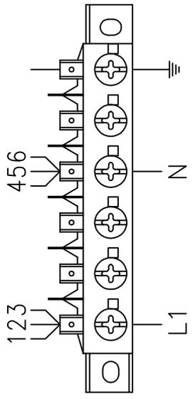
230V/3/50Hz 5450W 13.7A main cable 4X2.5mm<sup>2</sup>
