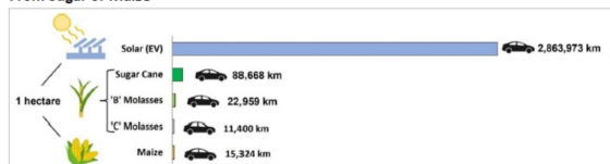
Figure 1: Vehicle Distance From 1 Hectare of Solar Energy or Ethanol From Sugar or Maize
